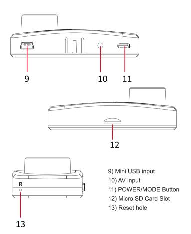
**NOTE:** Dash Cam supports up to 256GB Micro SD card. Class 10 Micro SD card is required.
