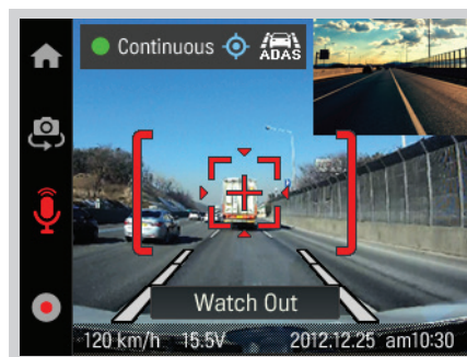
<2nd stage FCWS warning when fast approaching the vehicle ahead after initial warning was given>
