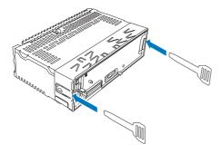
4 Install the sleeve into the dashboard and bend the tabs outward to fix the sleeve.
