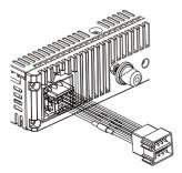
3 Connect the antenna and amplifier as illustrated, if applicable. You can connect the car audio to the amplifier through RCA-TO-RCA cables (not supplied).
