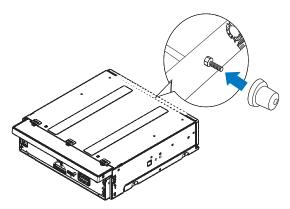
5 Install the sleeve into the dashboard and bend the tabs outwards to fix the sleeve. Slide the unit into the dashboard until you hear a click.
