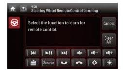
3 Tap an icon, for example, I◀◀, of which you want to assign the function to a button on the steering wheel.
