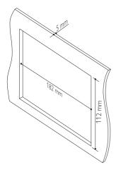
Since the unit cannot be used if the dashboard opening's slant angle is above 20 degrees, make sure that the horizontal slant of the car dashboard opening is between 0 and 20 degrees. Slide the unit into the dashboard until a click sound is heard.
