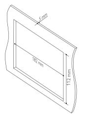
Since the unit cannot be used if the dashboard opening's slant angle is above 20 degrees, make sure that the horizontal slant of the car dashboard opening is between 0 and 20 degrees. **3** Slide the unit into the dashboard until a click sound is heard.
