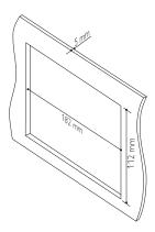
Since the unit cannot be used if the dashboard opening's slant angle is above 20 degrees, make sure that the horizontal slant of the car dashboard opening is between 0 and 20 degrees. 3 Slide the unit into the dashboard until a click sound is heard.
