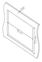
Since the unit cannot be used if the dashboard opening's slant angle is above 20 degrees, make sure that the horizontal slant of the car dashboard opening is between 0 and 20 degrees. 3 Slide the unit into the dashboard until a click sound is heard.
