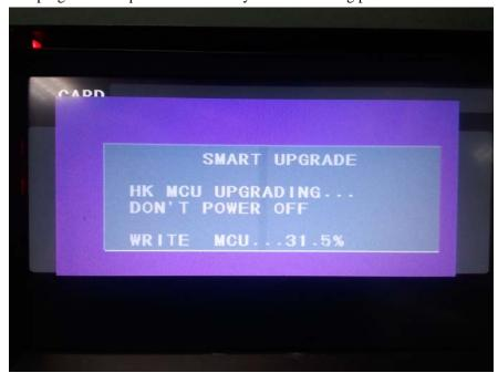
5. About 50 seconds, it will update complete ,the unit will reset automatically. Please pull out the U-disk before the unite enter the system. (If really delay to pull out the Udisk please wait for the second updating, don't put out the Udisk or power off the unite till update complete)
