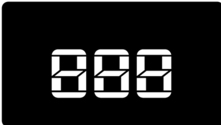
If the scanning failed, "000" will be shown on the display. Switch off the unit, check that all connections are correctly fitted and then restart the unit to re-scan.
