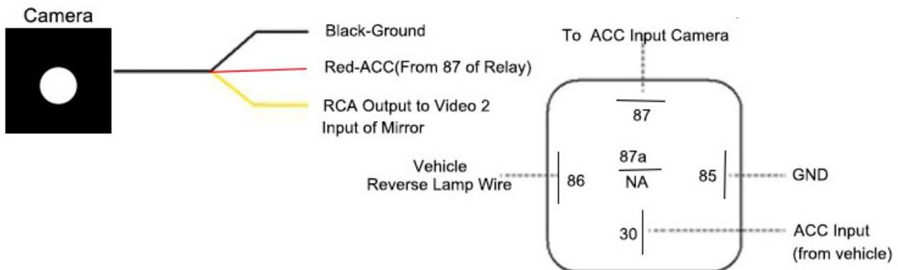
**Black (Ground)** – Locate a suitable location to ground (negative) the Black wire in the wiring harness. You may connect this wire to a factory ground point in the vehicle, or attach a ring terminal to the black wire and screw into the body of the vehicle. If you choose to screw into the body, clean the area of any paint or adhesives to allow for good metal-to-metal contact.
