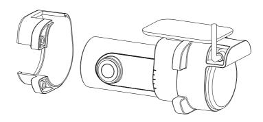
4. Screw the 2 security screws to secure the part using the provided key and rotate the DVR back back to the correct viewing angle
