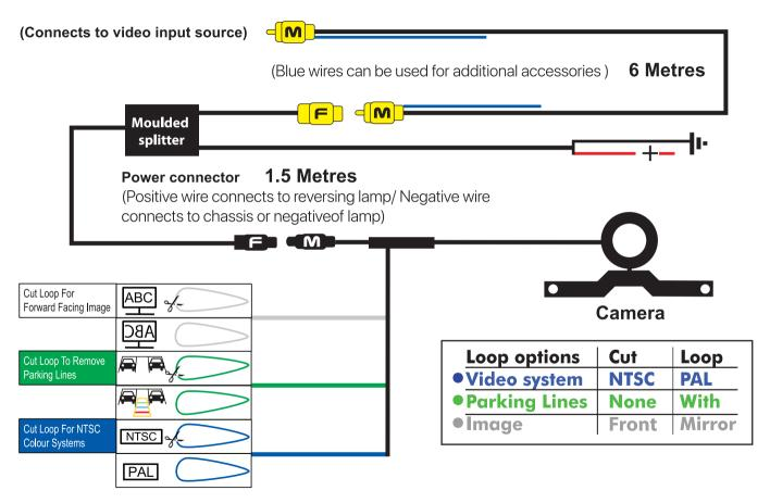
**Note:** When cutting loop wires make sure power to the camera is turned off. For CAN-BUS vehicles you will require a Gator GRCANFLT CAN-BUS filter. (Sold separately).
