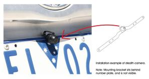
Where this is not possible there are other camera combinations that will suit your individual application. When mounting the camera, make sure that the camera does not cover any part of the license plate. Choose a position that does not impede the access/operation of the boot release or tailgate latch.
