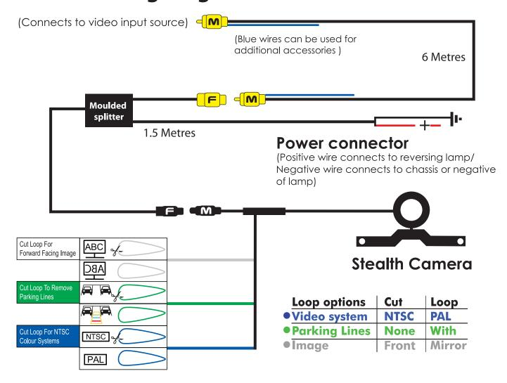
**Note:** When cutting loop wires make sure power to the camera is turned off. For CAN-BUS vehicles you will require a Gator GRCANFLT CAN-BUS filter (sold separately).
