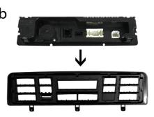
11c. Use the screws removed in Step 11a to reattach the button panel to the included trim piece, creating the new climate control button assembly for use in the installation.
