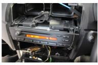
6. Disconnect the four (4) connections to the air conditioning panel
