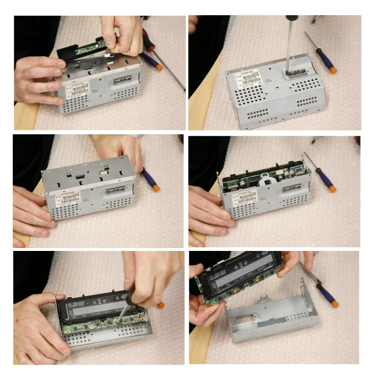
3. Insert the buttons into the new display if the buttons do not move freely we recommend filing out the openings on the display so the buttons move in and out without resistance. We also recommend adding a little foam to the buttons to reduce rattling.
