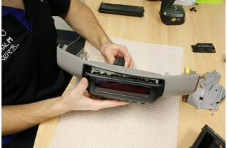
10. Thread the Compass cable through the backing plate into the facia
