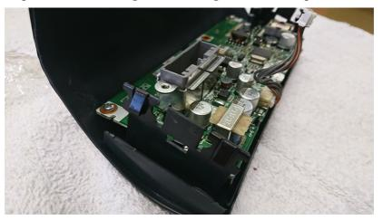
9. Insert the display into the lower mount of the Triton making sure that the Compass cable has been plugged in (for best results we recommend that this cable is extended so the compass can be attached to the top of the new stereo)
