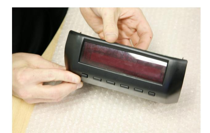
7. Remove the Lower panel out of the Triton as per manufacturers instructions, shave out the lower right corner to clear the capacitor and drill a hole (as shown) to clear other circuitry (if this is not done then it is possible to damage the main board on re assembly)
