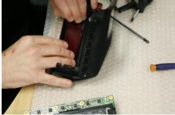
5. Screw the main board into the new display housing
