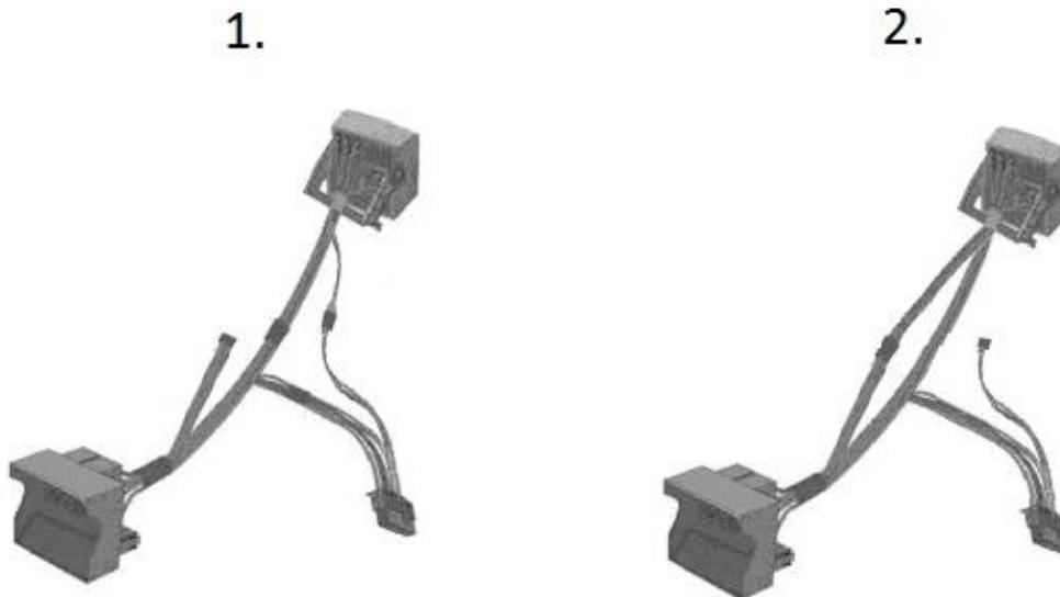
On fig. 1 the 4pin Molex from the radio side quadlock connects to the 18pin Gateway side connector, so the radio uses the Gateway Pro as a phone module. On fig. 2 the 4pin Molex from the radio side quadlock connects to the car side quadlock connector, so the radio uses the original phone module (if present). If the vehicle where the iGateway was installed, has a factory phone module, you need to install the 4-pin Molex connector as shown on fig. 2.
