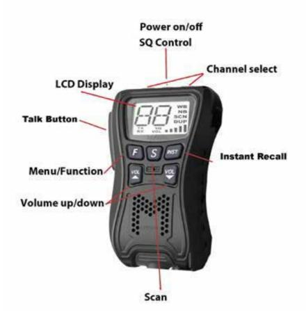
Note for Factory Reset: To reset the system. Press and hold the "F" Button while turning on the unit.
