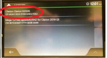
If the model number on the Licence matches the model number of the Unit, then the SD is not the fault cause. The unit will need to be assessed for repair at TDJ
