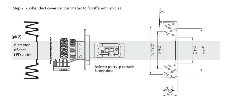
Step 3. Place collar in headlight housing. The rubber dust cover is then positioned onto headlight housing. The LED is then pushed in up against rubber dust cover and collar to seal.
