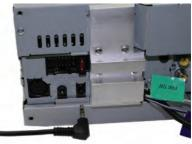
4. Connect the 14 way molex connector to the interface.
