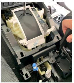
10. Remove the philips screw and lift the center console up, disconnect any cables
