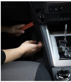
5. Remove the trim retaining clip by pushing the center in as shown
