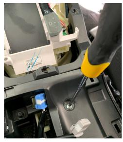
12. Unclip the trim from around the gear stick and place on a bench
