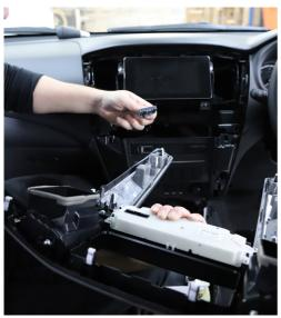
1. Unclip the surrounding trim on the dash using a panel remover
