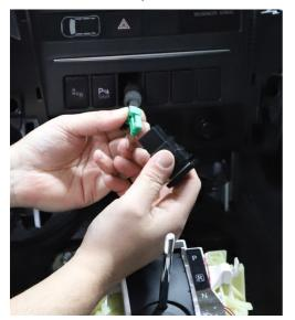
14. Run the switch connector up the back and through the switch hole
