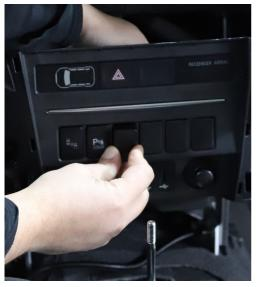
15. Plug the supplied switch in a push it into place
