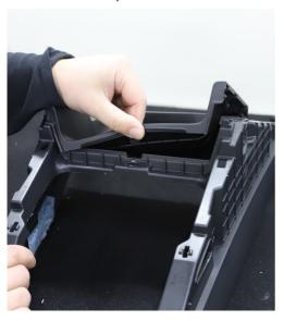
17. Install the new trim so the cable is out the back for easy connection
