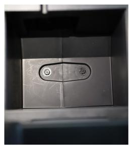
11. Remove the 2x 10mm bolts to release the trim around the gear stick
