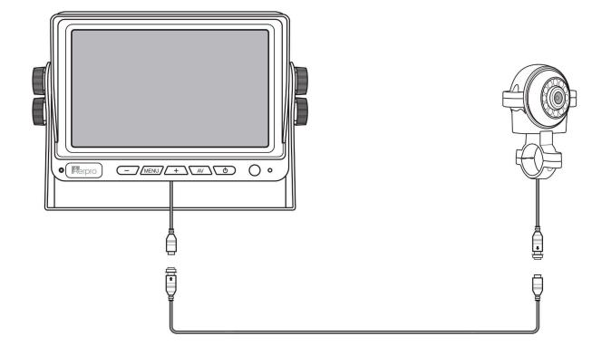
**Note:** This camera is supplied as a camera only with a 50cm cable. Extension cables and monitors are sold separately. The following wiring diagram illustrates the complete camera system. **Note:** Extension cables available AVEC3, AVEC5, AVEC10, AVEC15 and AVEC20.
