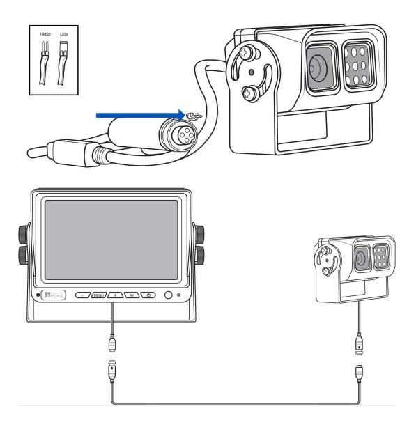
**Note:** This camera is supplied as a camera only with a 50cm cable. Extension cables and monitors are sold separately. The following wiring diagram illustrates the complete camera system. **Note:** Extension cables available AVEC3, AVEC5, AVEC10, AVEC15 and AVEC20.
