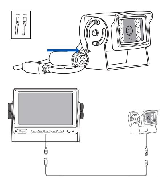
**Note:** This camera is supplied as a camera only with a 50cm cable. Extension cables and monitors are sold separately. The following wiring diagram illustrates the complete camera system. **Note:** Extension cables available AVEC3, AVEC5, AVEC10, AVEC15 and AVEC20.
