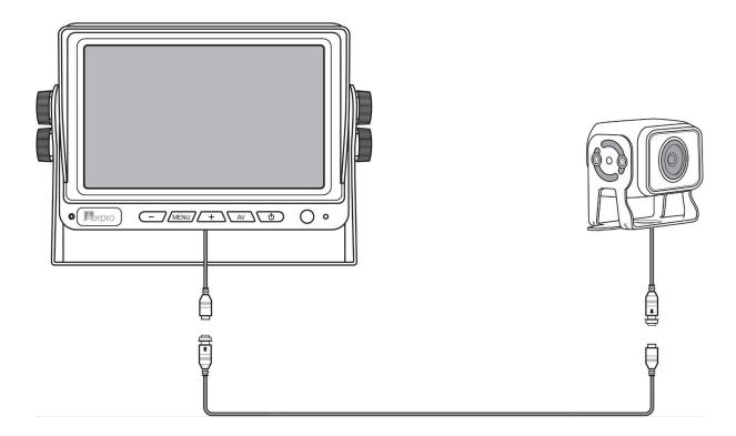
**Note:** This camera is supplied as a camera only with a 50cm cable. Extension cables and monitors are sold separately. The following wiring diagram illustrates the complete camera system.
