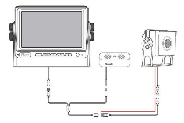
**Note:** This camera is supplied as a camera only with a 50cm cable. Extension cables and monitors are sold separately. The following wiring diagram illustrates the complete camera system. **Note:** Extension cables available AVEC3, AVEC5, AVEC10, AVEC15 and AVEC20.
