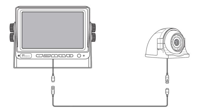
**Note:** This camera is supplied as a camera only with a 50cm cable. Extension cables and monitors are sold separately. The following wiring diagram illustrates the complete camera system.
