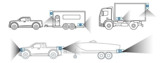
**Note:** Above images are examples of where the camera can be installed.
