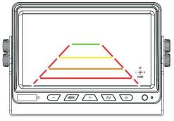
Press the Confirm key in the middle of the key and move it counterclockwise to the corresponding adjustment node, as the white dot shown in the above picture.
