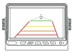
5. Press the middle confirm button to save the Settings after the adjustment finish. Note: If you do not press the confirm button after adjustment, the data will not be saved. After power off and restart, the data will return to the defaulted one.
