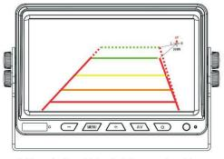
After moving the node to be adjusted, press up, down, left, or right to move the location, as shown in the figure, the node in the upper right corner moves upward and widens the range of overlay line.
