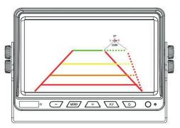
After moving the node to be adjusted, press up, down, left, or right to move the node, as shown in the figure, the node in the upper right corner is moved to the right, and the range of, overlay line is widened.
