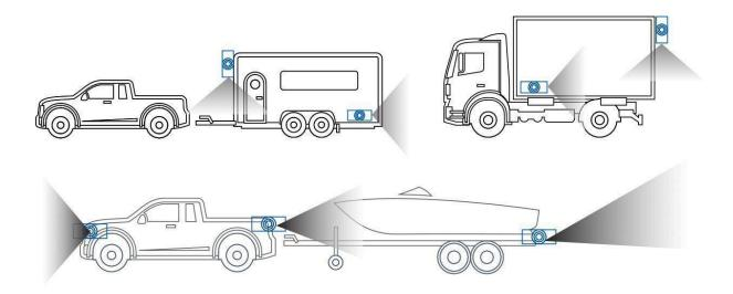
Note: Above images are examples of where the camera can be installed.
