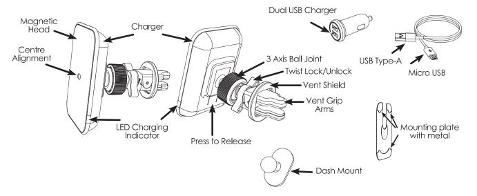
Note: Dash Mount can be used as an alternative to the Vent Mount. Loosen ball joint collar. Pull ball joint out of socket. Place collar over dash mount ball. Push dash mount ball back into socket. Tighten collar.
