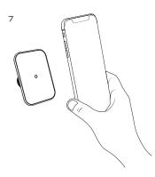
Once the mounting plate is fitted on the back of the phone or inside phone cover, align the centre of your phone with the circle on the holder to charge. LED charge indicator will turn red while charging. If indicator flashes red, reposition phone for better connection.
