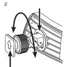
Arrow faces upwards when mounting to charger. Twist clockwise to loosen 3 Axis ball joint, twist anti-clockwise to tighten
