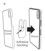
The mounting plate sticks to the back of the phone directly. Remove protective adhesive cover to adhere to phone. Then the phones cover, covers the plate.
