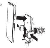
Place phone in holder and press arms inwards for secure grip on phone. Adjust sliding head to appropriate position. LED charge indicator will turn red while charging. If indicator flashes red, reposition sliding head for better connection.
