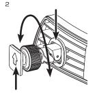
Arrow faces upwards when mounting to charger. Twist clockwise to loosen 3 Axis ball joint, twist anti-clockwise to tighten.
