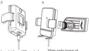
Insert Micro USB end of the cable into the base of the wireless charger and USB Type-A end in to a USB charger
