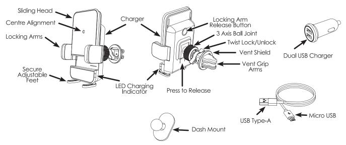
Note: Dash Mount can be used as an alternative to the Vent Mount. Loosen ball joint collar. Pull ball joint out of socket. Place collar over dash mount ball. Push dash mount ball back into socket. Tighten collar.
