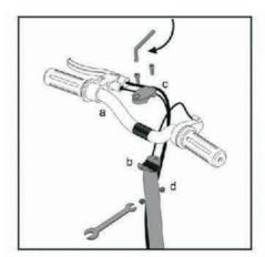
3. Align the handlebar (a) on the steering handle tube clamp (b) install the handlebar clamp and hardware (c & d) and tighten evenly and securely with the 5mm hex wrench and one 10mm wrench.
