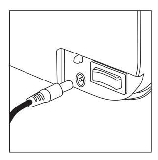
1. Make sure that the switch is in the off position before plugging in the charger. Insert the charger into the charging input on the scooter on the right side of the battery case.
