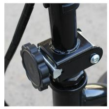
3. Pull the handlebar to the upright position and tighten the round knob to engage the clamp so the handlebar is secure in the upright position.
