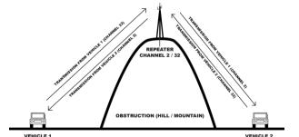
VEHICLE 1 RADIO IN DUPLEX MODE ON CHANNEL 2
