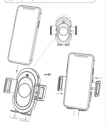
**NOTE:** Due to different phone sizes, the wireless charging contact area may vary. Adjust the feet by pulling down to allow alignment between the phone and the wireless charger contact area.
