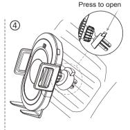
Press button on vent clamp to open grip arms, then place mount on vent. Release button to secure on vent
