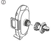
Place the nut over the ball on the vent mount. Press ball into charging base.
