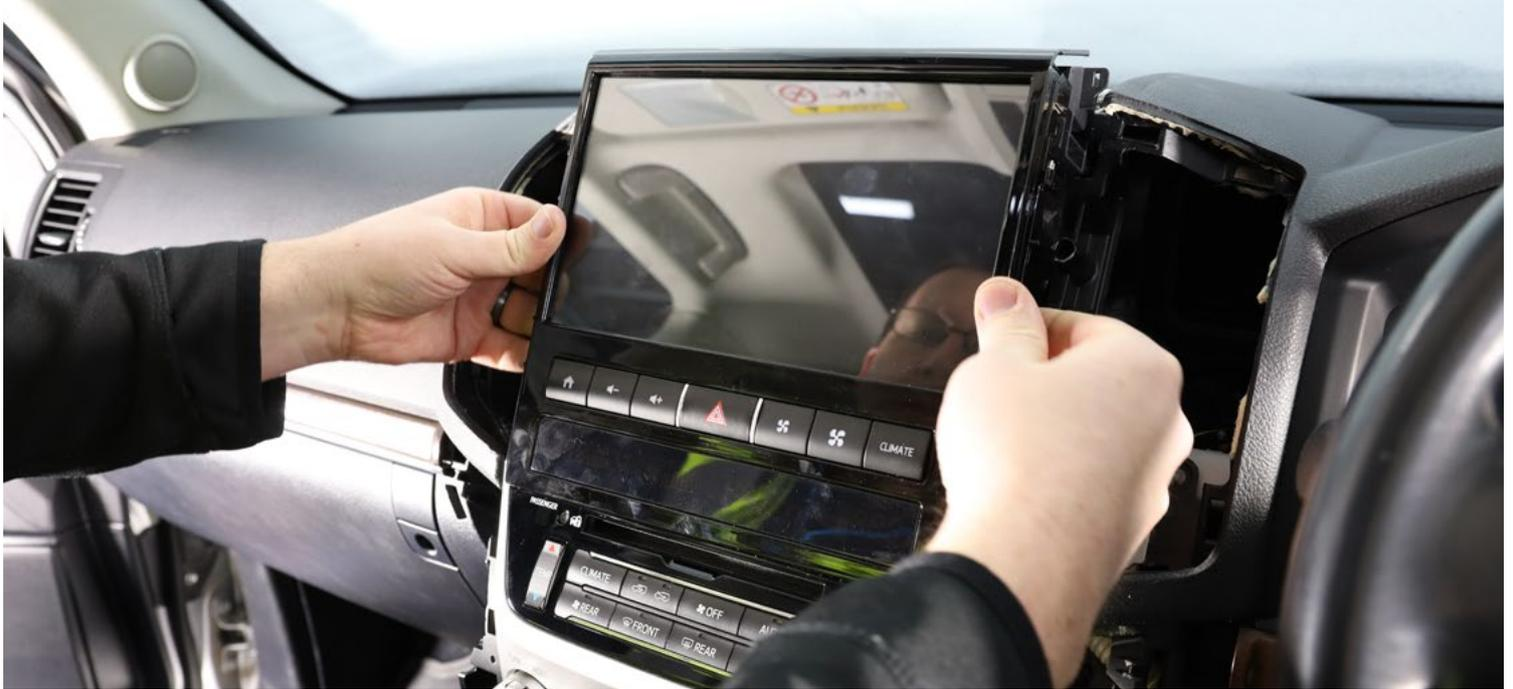
The dash top panel can be replaced by first connecting the original light sensor harness and then clipping it into place by firmly pushing it down with even pressure by hand.
