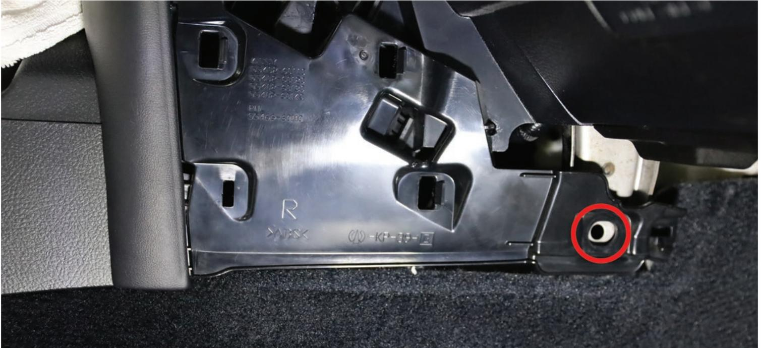
Remove the panel with the engine start / stop button by pulling it firmly on an angle toward yourself as indicated in figure 2.
