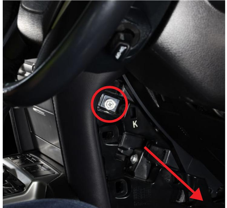
The panels by the drivers left knee and the passengers right knee can both be clipped back into place
