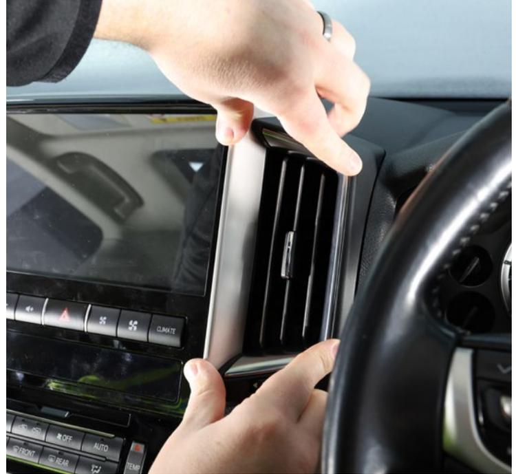
The pocket below the original stereo can be replaced by firmly pushing it into place with even pressure by hand. (You may require the harnesses to be reconnected before replacing this panel).
