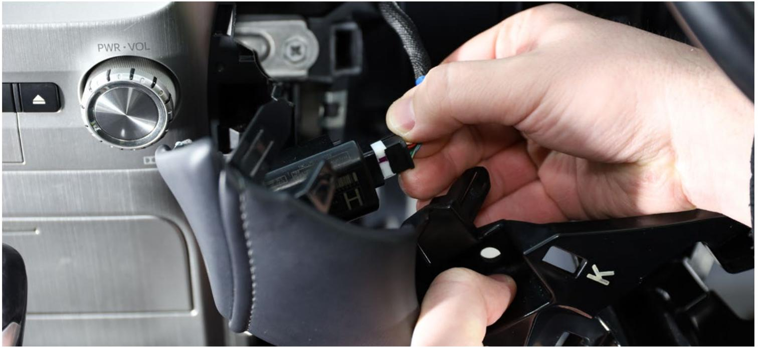
Repeat the process on the opposite side, remove the panel located by the right knee of the passenger by pulling it firmly toward yourself. Place this panel aside.
