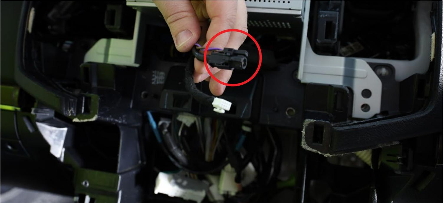
Hazard switch and climate display harness (white 8-pin plug) (2)
