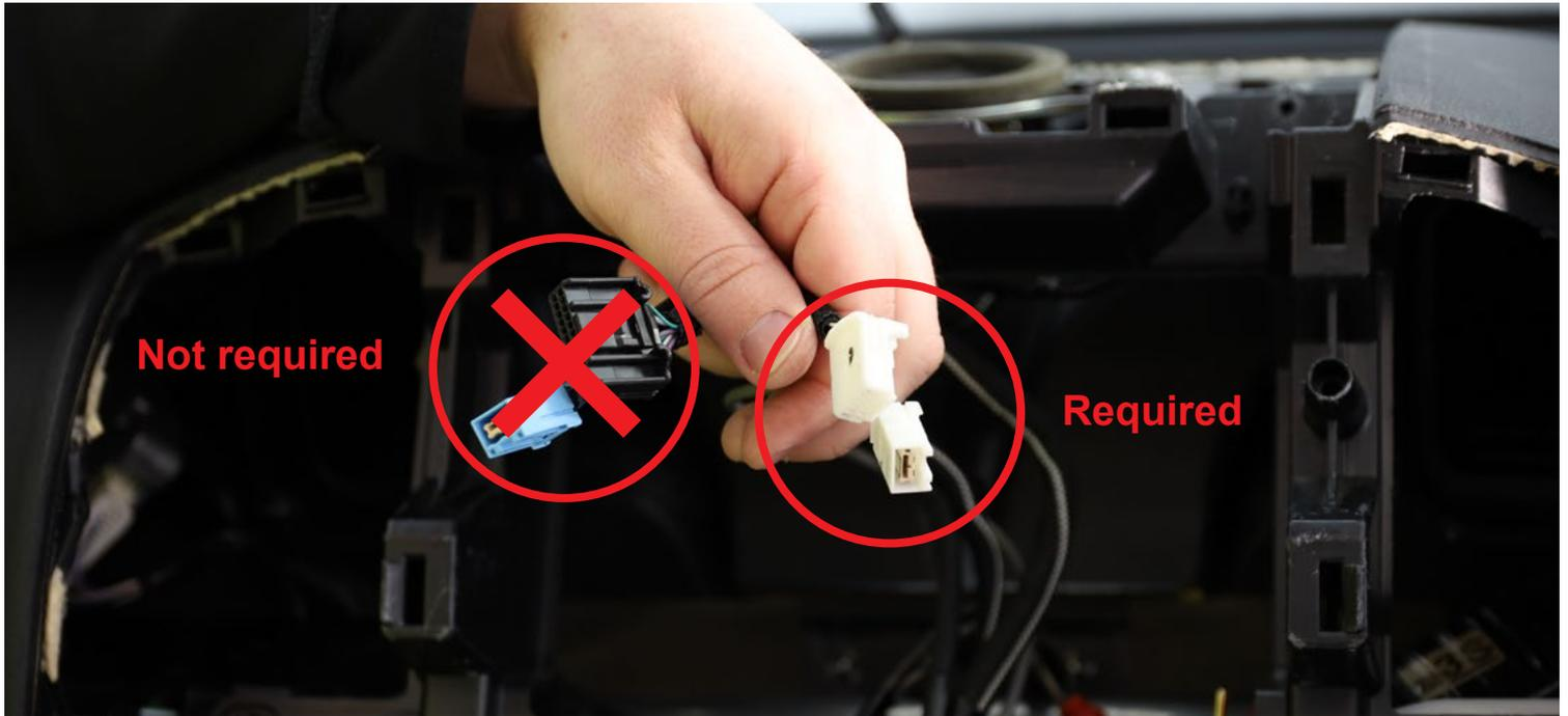
For the Australian region, the **360 camera plug is white or black and not blue.** If your vehicle has a 360 camera connector like Figure 9 then before continuing you will need to use the blue 360 camera adaptor shown in Figure 10.
