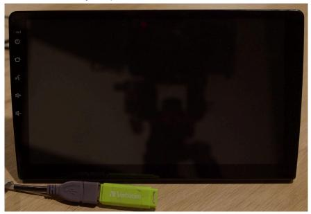
Once the USB is inserted, turn on your vehicle to accessory. The head unit will start on a black screen and may flash white. This means the head unit will begin updating its firmware.
