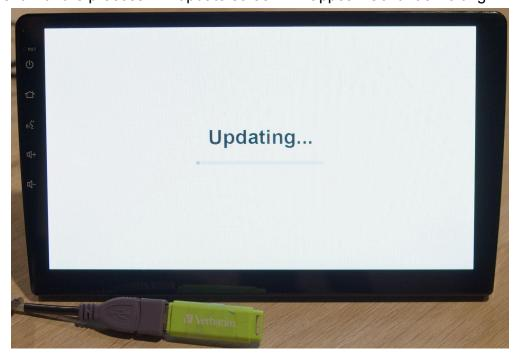
Once the headunit is finished updating, it will reboot and show the home screen/radio. **Disconnect the USB device & Turn off the car, wait 30 seconds then turn it back on**. Then you can check the date number to make sure it has updated successfully and you may change the settings to your taste.
