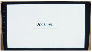
Once the head unit is finished updating, it will show the home screen/radio but will be **slightly dim** (like the image below). This is OKAY. Once you see this screen, you can Disconnect the USB device & Turn off the car, wait 30 seconds then turn it back on. Then you can check the date number to make sure it has updated successfully and you may change the settings to your taste.
