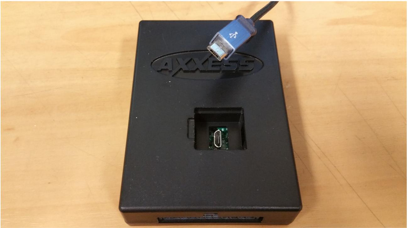
Insert a micro USB into the socket and plug the other end to the computer.
