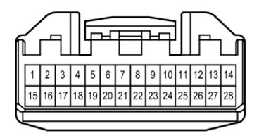
This is the pin view of the connector in the vehicle
