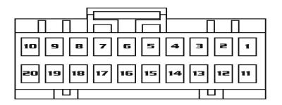
This is the wire view of the connector in the vehicle
