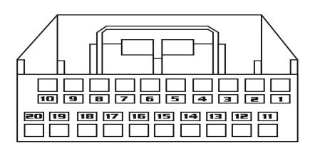
This is the pin view of the connector in the vehicle
