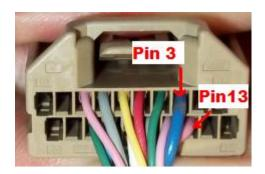
This is the wire view of the connector in the vehicle
