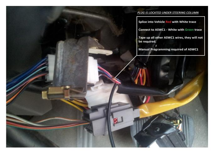
\*\*\*\* DO NOT PLUG ASWC1 PATCH LEAD INTO HEAD UNIT UNTIL LAST STEP \*\*\*\*
