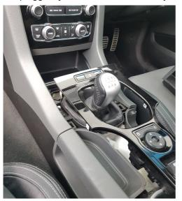
1. Unclip the trim around the gear stick directly upwards with a panel remover
