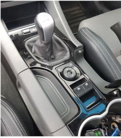
3. Remove the 2x philips head screws located at the front of the pocket
